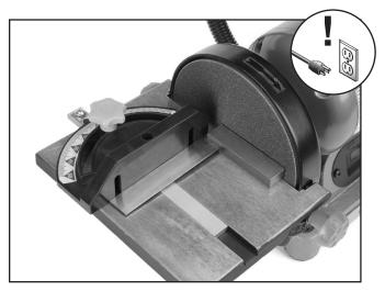
Figure 7. Squaring the miter gauge.
